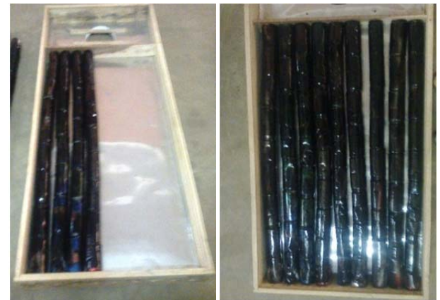
Fig. 6: Fixing of cans, tempered glass, induced fan
