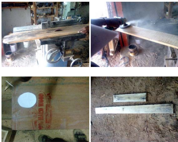
Fig. 3: Step wise process of preparing a wooden frame
